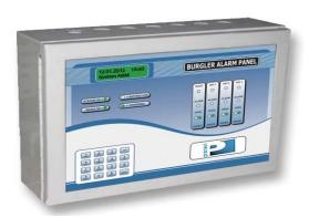
4200 Series panel is Fire cum Burglar Alarm panel with Auto Dialer. The Panel have 6 Zones that are split into 2 Fire, 1 Night and 3 emergency zones. Panel have unique feature that all burglar zones also work like fire zone and gives OPEN alert at the time of broken wire, this will stop the false alarm due to broken wire. Panel also have Auto Dialer feature with 10 telephone numbers store capacity and also have 2 different type of messages for Fire & Burglar events.
